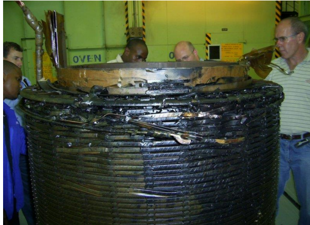
Burning in the vicinity of the top core earth strap
