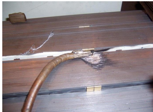
Burning in the vicinity of the top core earth strap
