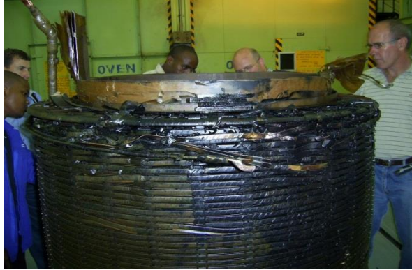
Figure 36 Shows the damage on the HV winding
