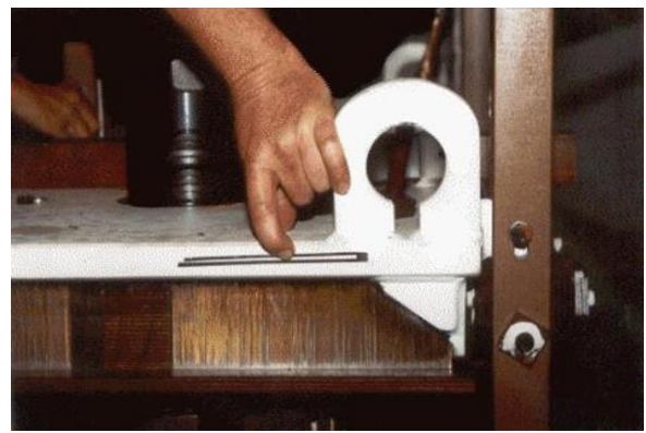
Figure 17 Showing the point on the Resistor bank where the Overheating was occurring
