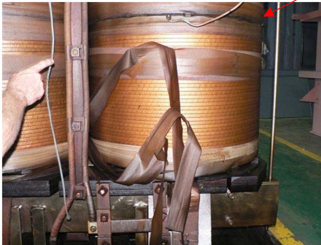
Extensive deterioration of the LV and Tap changer Leads
