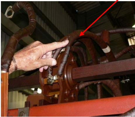
Extensive deterioration of the LV and Tap changer Leads
