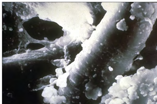
Figure 3: Electron microscope picture of paper aged in oil (Acid value 0,15 mg/kg) Courtesy of SD Myers
