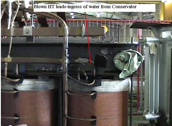
Figure 11-Point of failure
