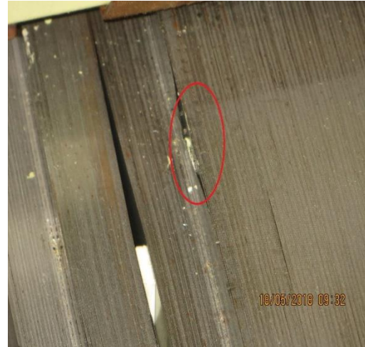
Figure 3: Secondary fault observed on the Core
